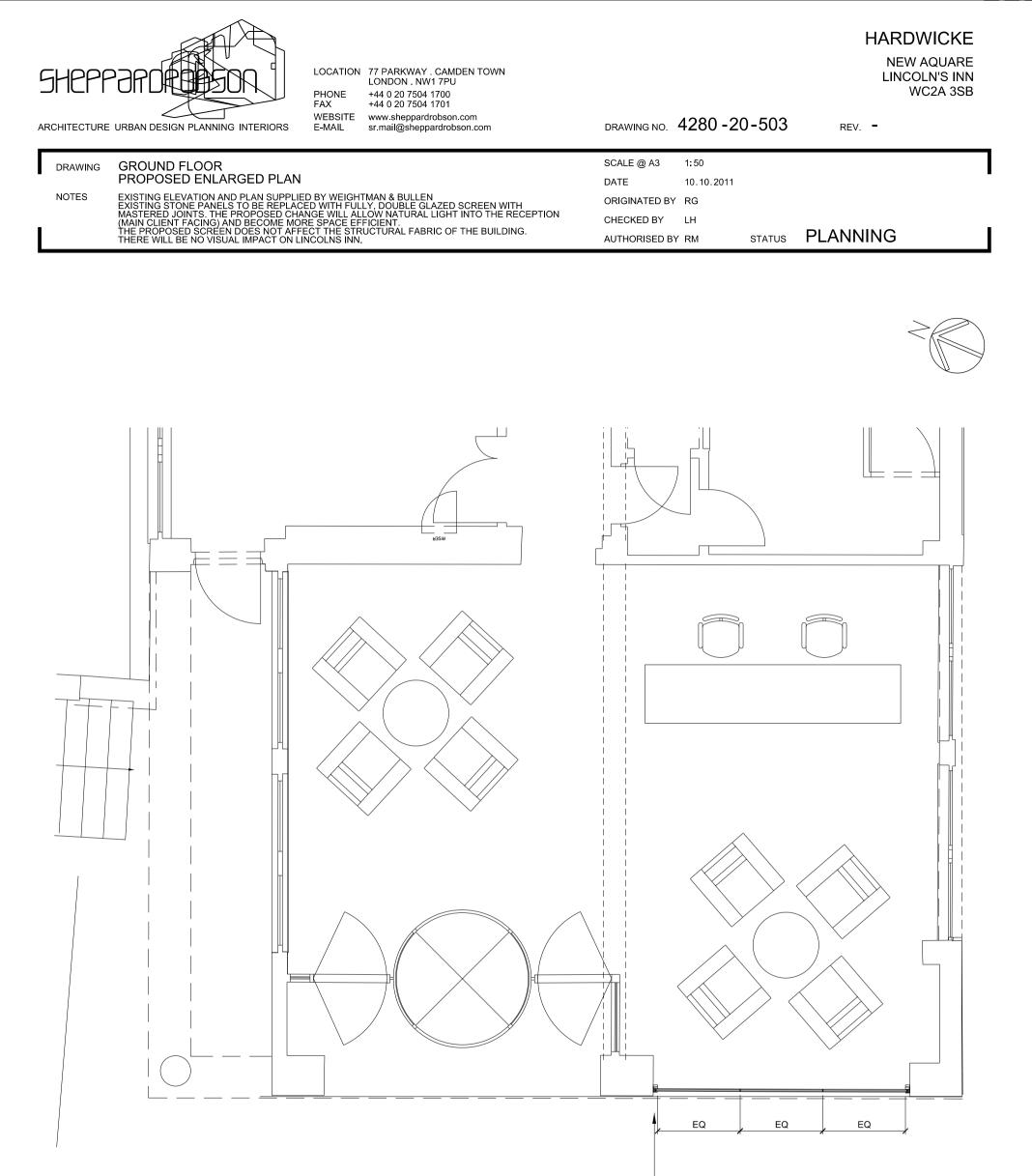
NEW FULL HEIGHT DOUBLE GLAZED SCREEN WITH 50MM – STAINLESS STEEL PERIMETER FRAMEWORK TO MATCH EXISTING. SURROUNDING NATURAL EXISTING STONE TO BE CAREFULLY RETAINED. MANIFESTATION WILL BE APPLIED TO THE GLAZING
