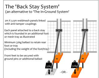
5.5.7. The panel should be secured in the edge holes of the front foot and one foot per two panels should be further secured using ground pins. This system will withstand occasional knocks by machinery and is not easily relocated.
