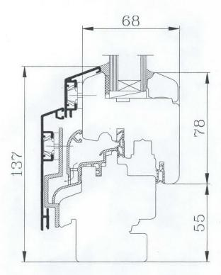
All window systems are manufactured in an ISO9001 registered factory and meet the performance requirements of BS6375, BS5268 and BS5368 for wind resistance, weather-tightness, operation, strength and air-permeability. Windows are also tested to BS7590 for enhanced security.
