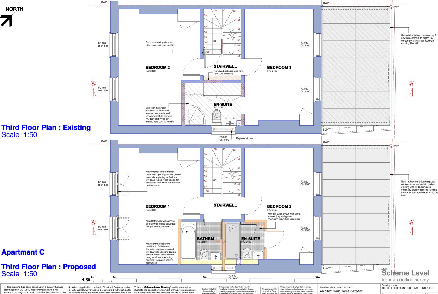
Third Floor Plan: Proposed Scale 1:50
