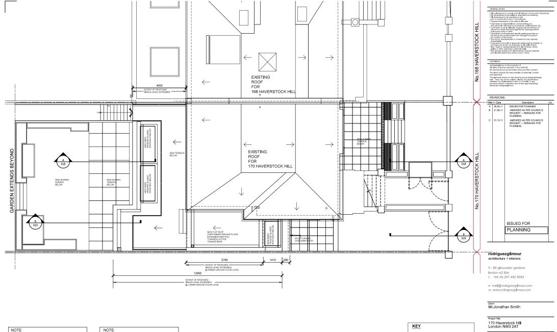
All New glazing to be energy efficient. New Aluminium Framed Glazed Sliding Door and Fixed Glass Pane to be glazed to provide a min 'U' value of 2.0W/m2k, utilising 28mm DGU: 6mm clear toughened safety outer glass, in 14mm Black Silicone Space Bar hermetically sealed double-glazed units with low 'E' coating for improved thermal efficiency, 8mm laminated soft coat Low e inner pane.
