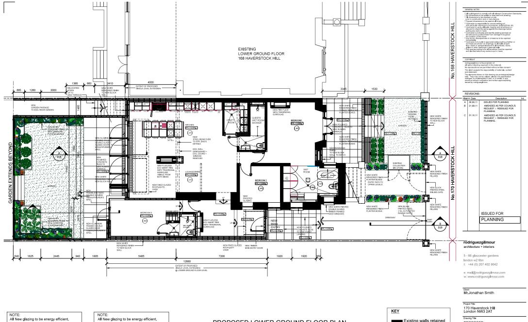
New Aluminium Framed Glazed Sliding Door and Fixed Glass Pane to be glazed to provide a min 'U' value of 2.0W/m2k, utilising 28mm DGU: 6mm clear toughened safety outer glass, in 14mm Black Silicone Space Bar hermetically sealed double-glazed units with low 'E' coating for improved thermal efficiency, 8mm laminated
