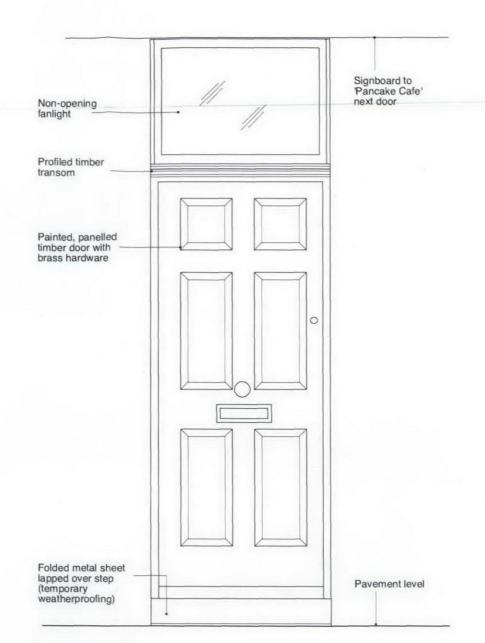
Existing Elevation Scale 1:20 @ A3
