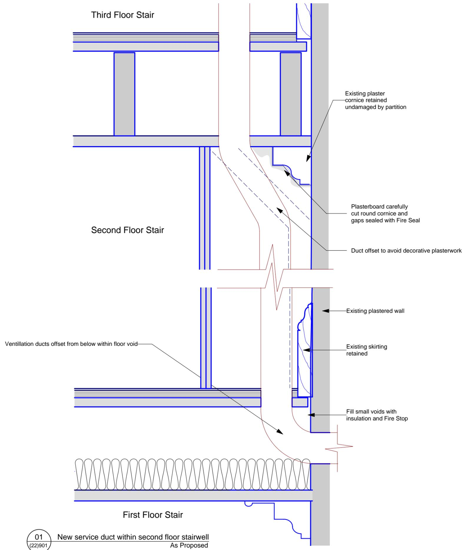
01 (22)901 New service duct within second floor stairwell As Proposed
