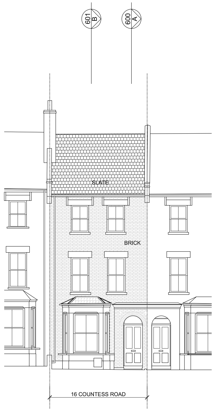
EXISTING FRONT ELEVATION
