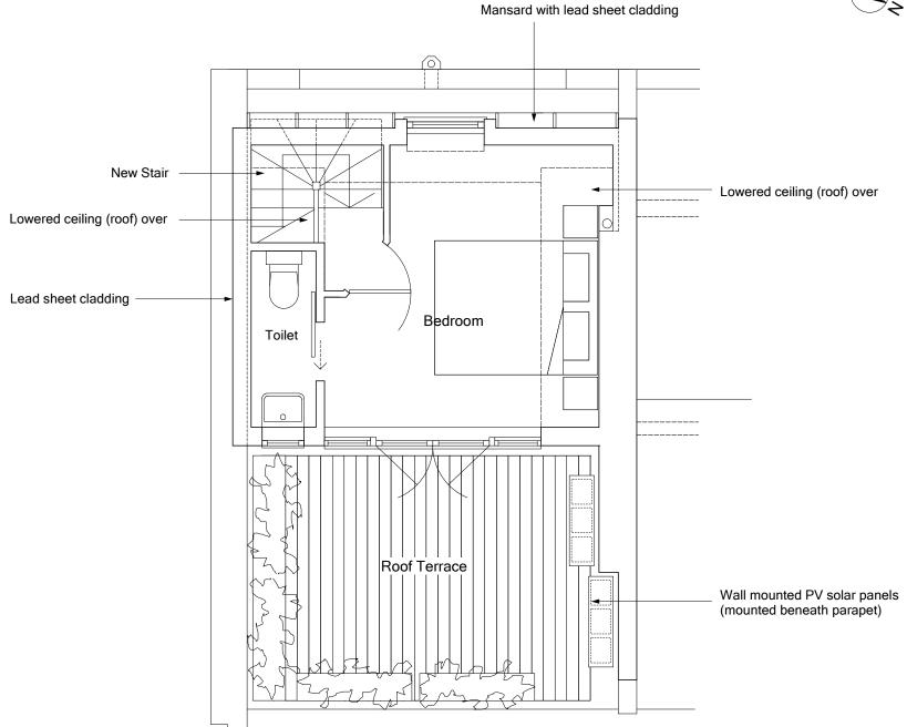
Proposed Second Floor Plan scale 1:50@A3
