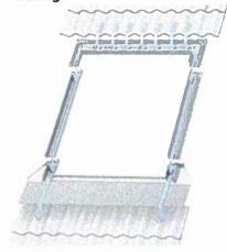
Our range of flashings will provide a weathertight seal between your roof window and roofing material
