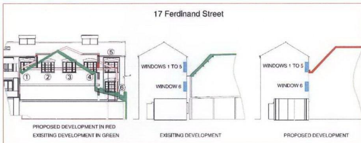
Figure 3: 25 Degree daylight results for 17 Ferdinand Street
