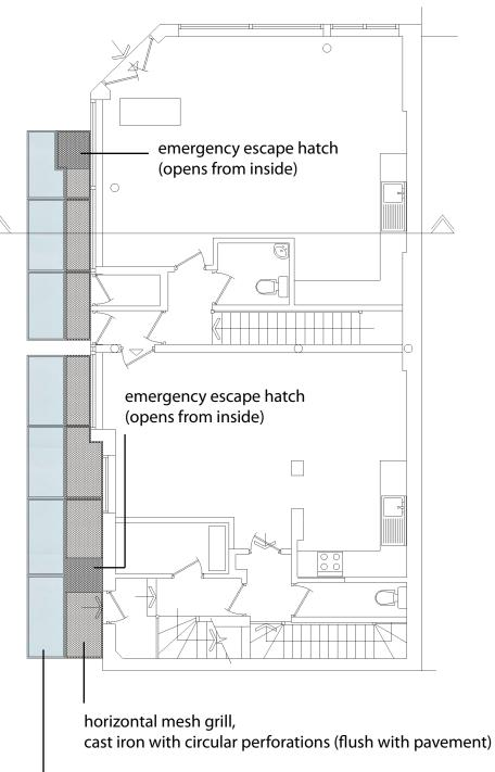
32 mm toughened, opaque walk-on glass sandblasted for anti-slip (flush with pavement)
