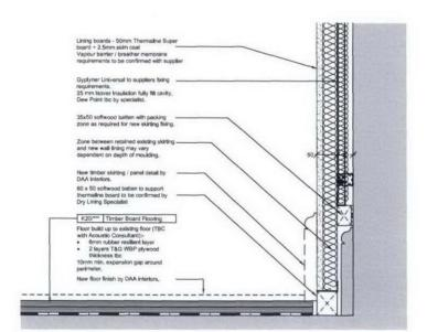
Typical External Wall Section - Detail E
