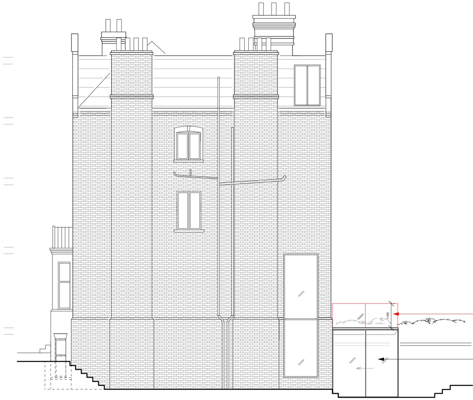
New glass balustrade to replace the original solid one, height as before
