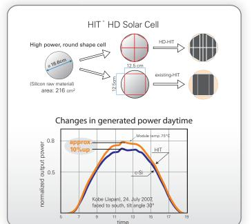
The HIT cell and module have very high conversion efficiency in mass production.
