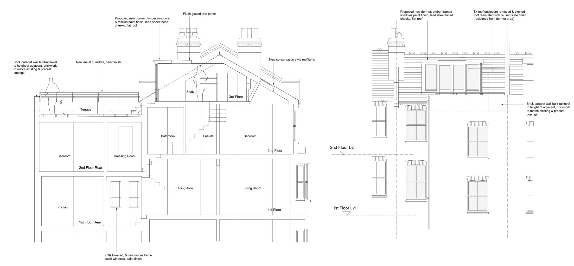
Proposed Section A-A scale 1:50@A3
