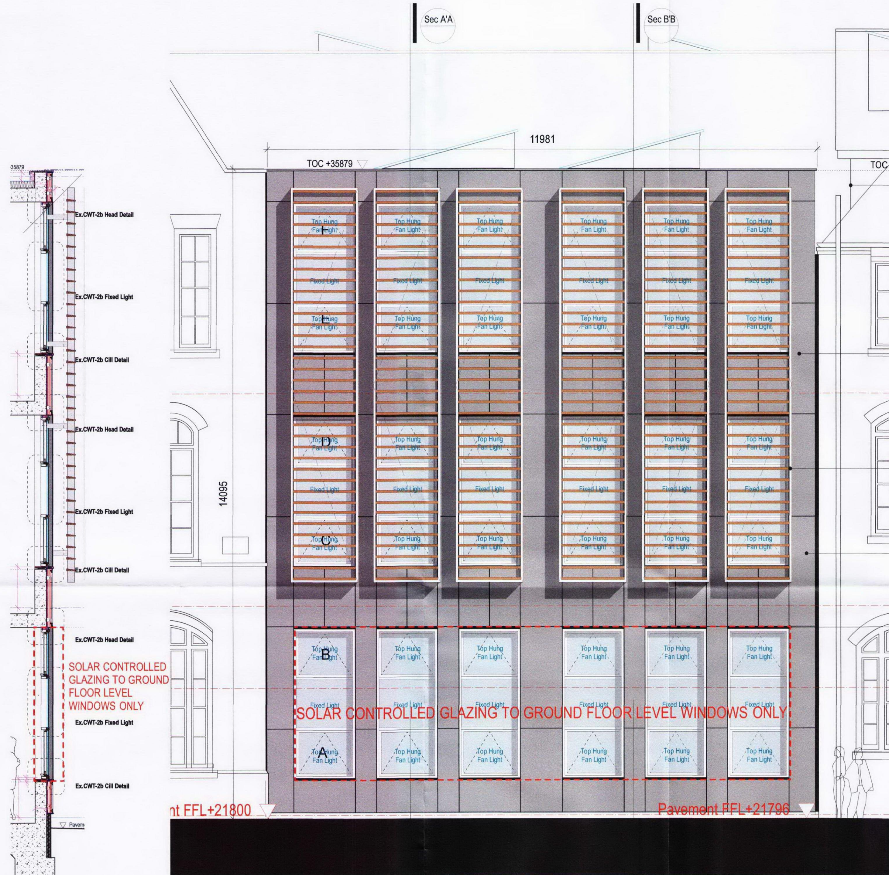
Ex.CWT-2b Alternative Glazed Curtain Walling Type, Section A/A 1.50
