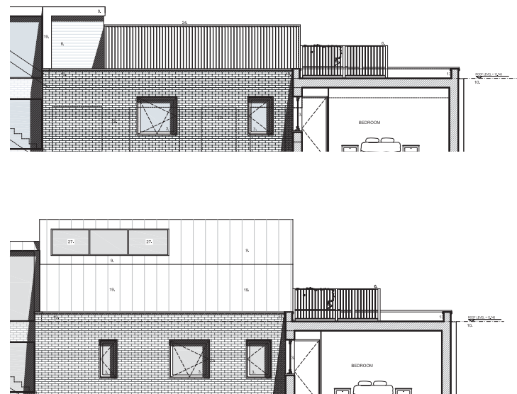
North Elevations: 2011 scheme (below) and 2012 (bottom). Care has been taken when redesigning the roofscape to protect views from street level / ground level. The zinc-clad extension stops at the height of the previously-proposed terrace fence.
