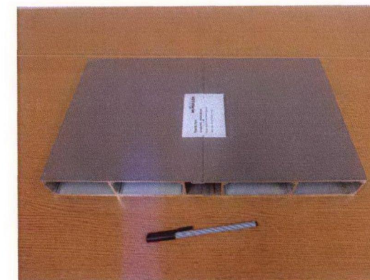
Sample SA044 - Material reference HSO.C01 Office building horizontal fins
