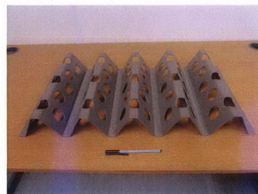
Sample SA041 - Material references AB.F01, HSO.W03 Affordable Block fins to Hampstead Road, office plant enclosure screen
