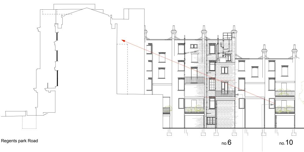
Sand blasted frameless glass privacy screen 1800mm from deck - steel supports to terrace side facing North.
