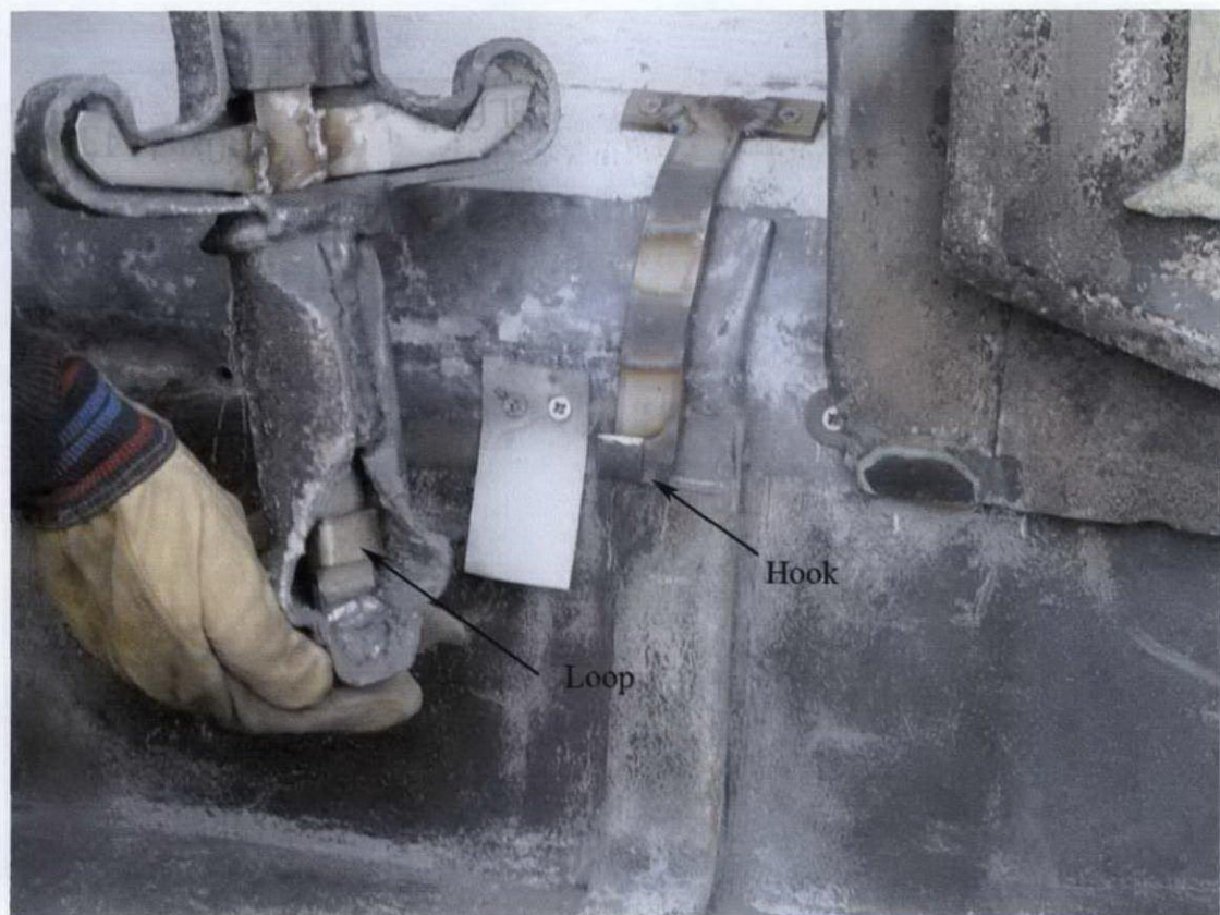
Figure 7. Close-up of bottom sword fixing
