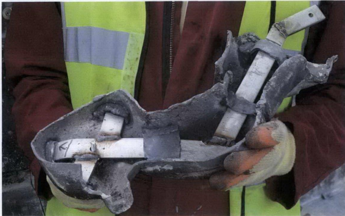
Figure 10. Right-hand swag with armature
