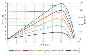
Exellent performance under weak light conditions: at an irradiation intensity of 200 W/m² (AM 1.5, 25 °C), 95.5% or higher of the STC efficiency (1000 W/m²) is achieved
