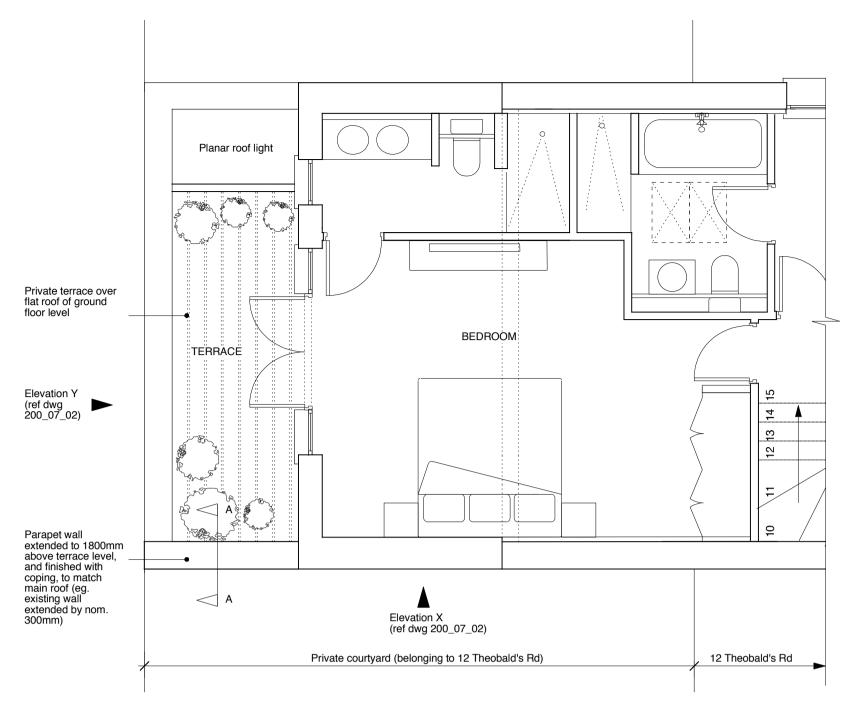
PROPOSED PART-1ST FLOOR PLAN Scale 1:50@A3 Refer to Campbell Architects' dwg 1176\_15\_202 for ful details (Planning Ref 2011/1302/P)
