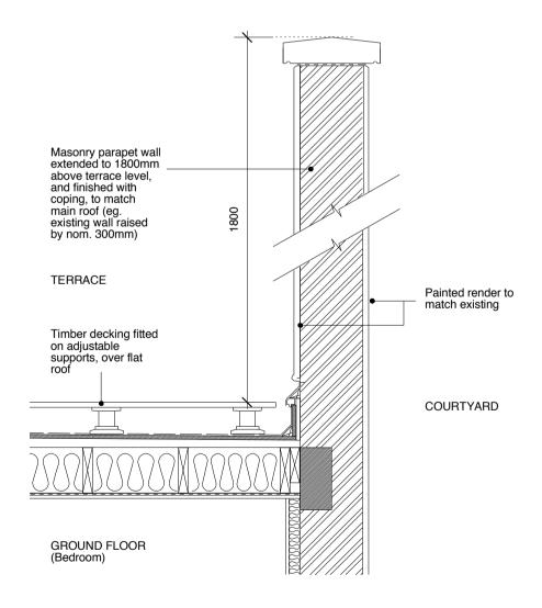
SECTION A-A: PARAPET WALL/PRIVACY SCREEN DETAIL Scale 1:20@A3
