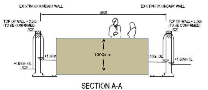
**Demolition and Excavation:** Area in highlighted in tan to be excavated to same level as existing lower ground flat patio. NE steps to be removed or blocked in as part of new retaining wall. Existing brick retaining wall to be removed. Approximately 22 square meters of dirt to be removed. (6475mm X 3500mm X 1000mm). Retaining walls with drainage to be installed.
