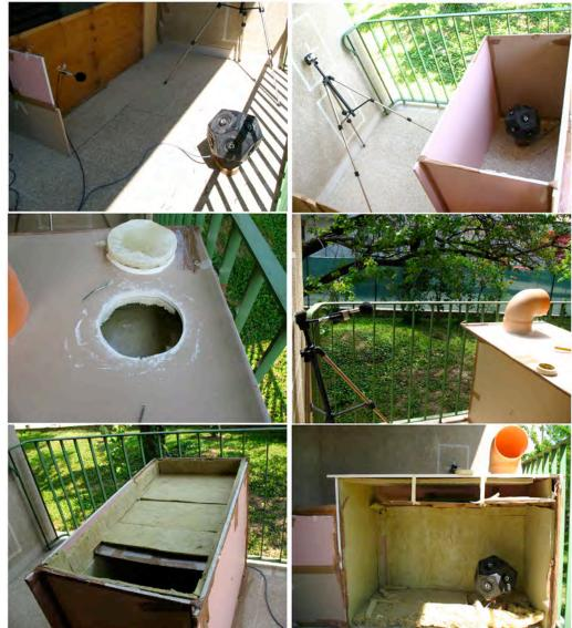
6.1.4 Fig showing enclosure construction and testing phases.
