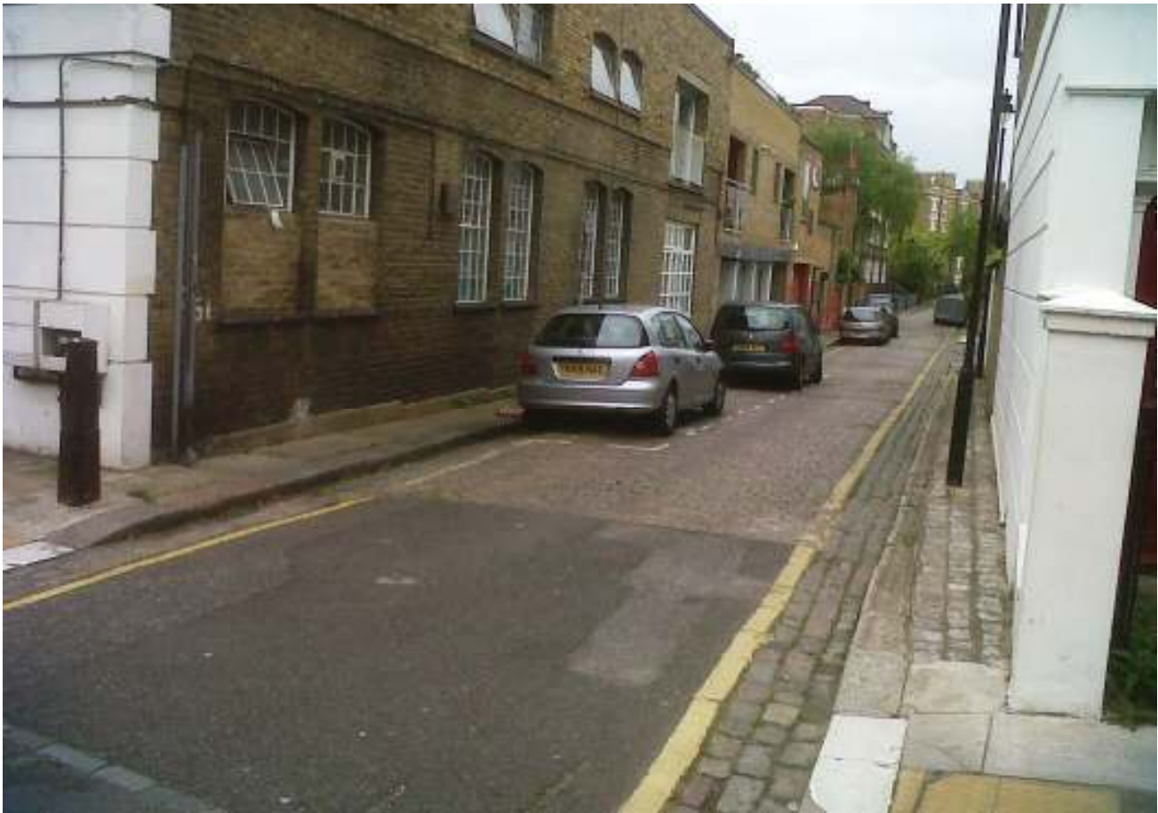
Photo 1 Junction of Rochester Place and Wilmot Place with 3 parking bays outside No 55 Note 1 At eastern end of parking bay, the road is 4.4m, parking bay 1.9m and net carriageway 2.5m
