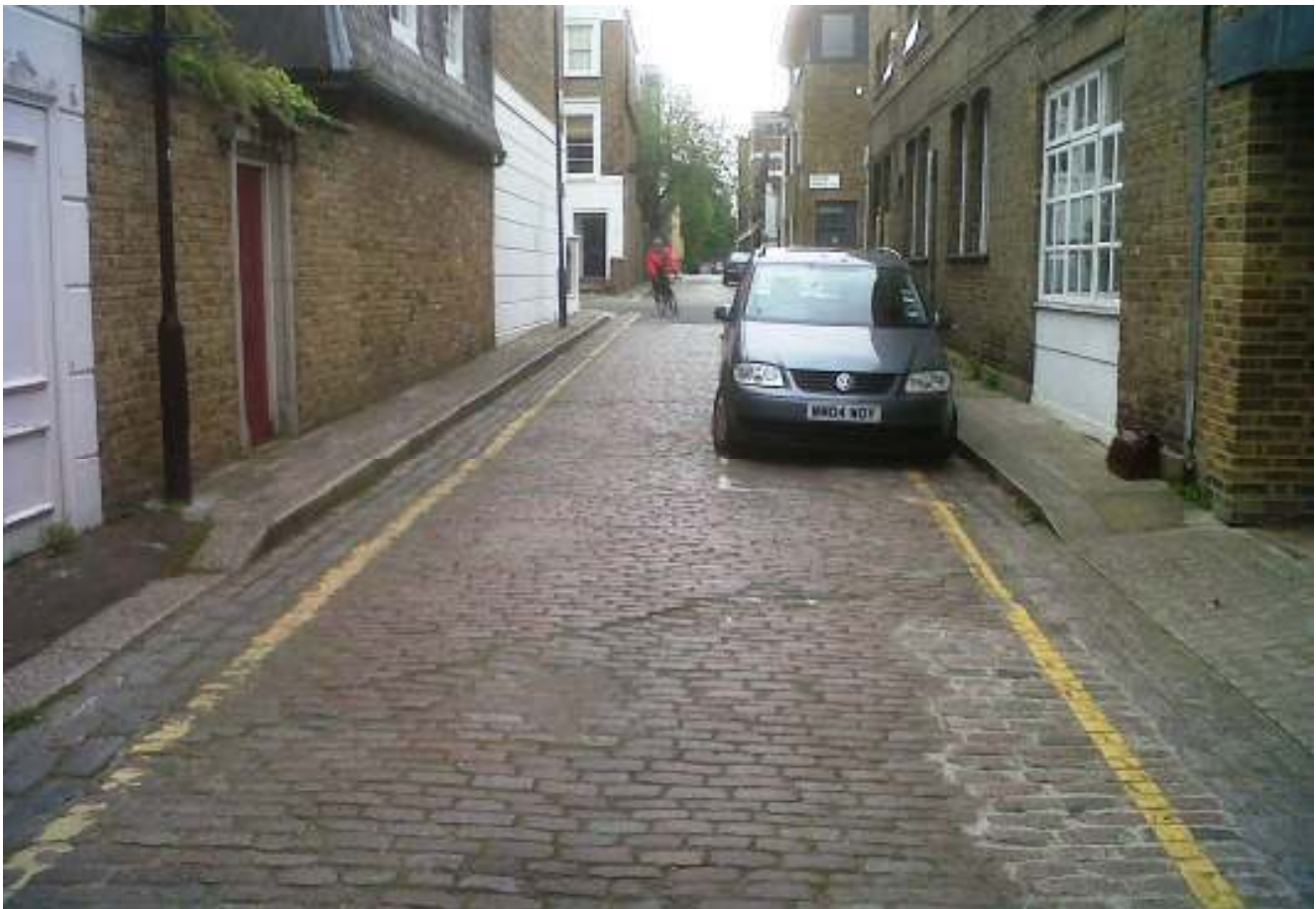
Photo 2 Western end of parking bays outside No 55 looking back to junction with Wilmot Place to east Note 1 At western end of parking bay, the road is 4.35m, parking bay 1.95m and net carriageway 2.4m
