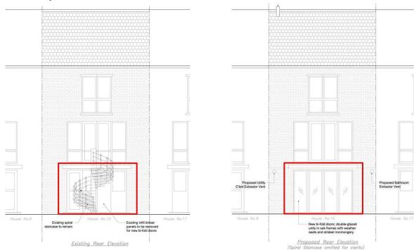
The proposal is to remove the existing window, single leaf door and timber infill panels at the rear of the property at Ground Floor and to replace with new bi-folding doors. The design of the new doors will be in keeping with the existing scale, nature, materiality and appearance, without deterring from the local context.
