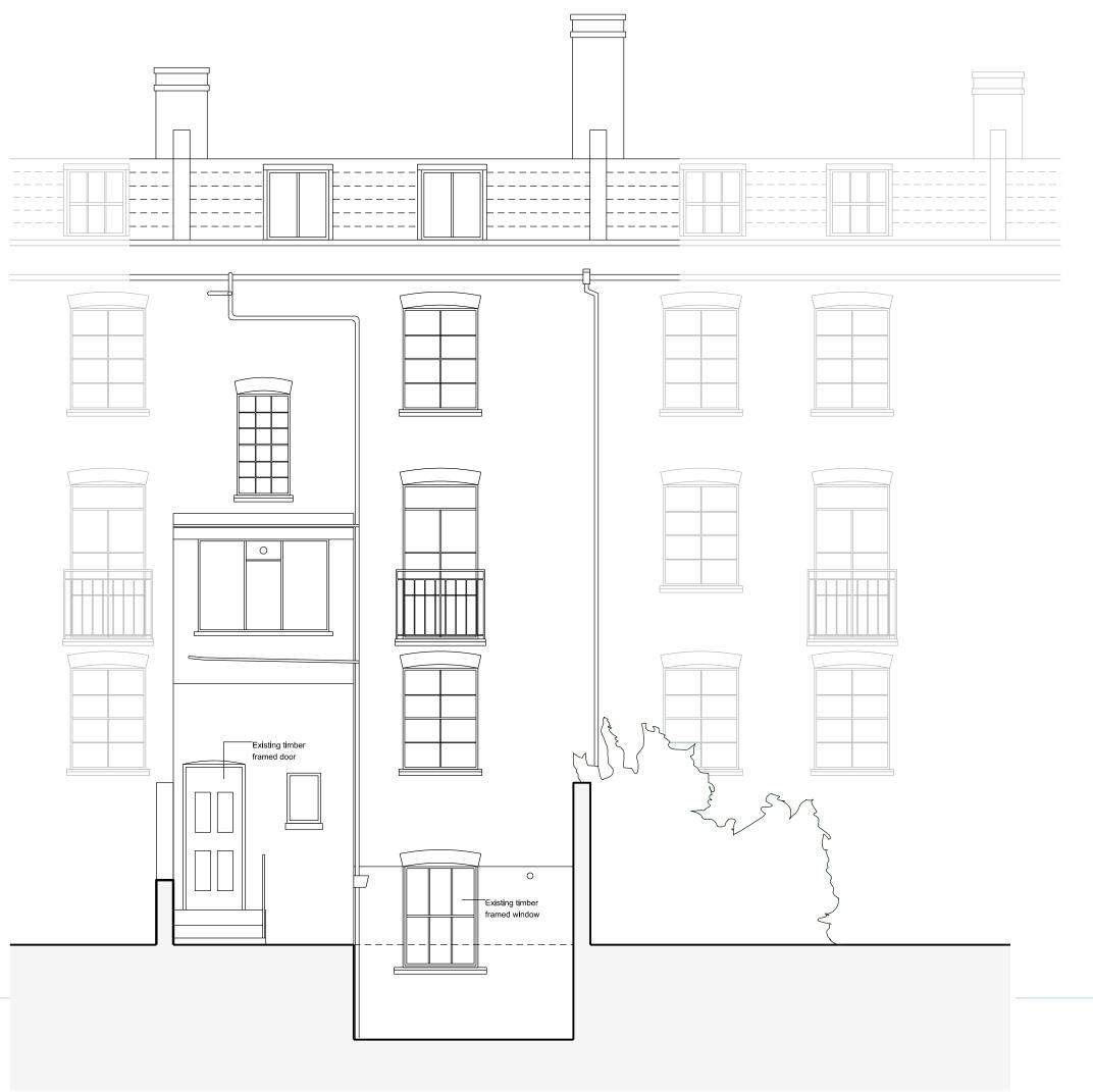
Existing East Elevation Scale 1:50 @ A3
