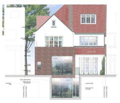
REAR: The design of the rear extension remains as approved in the application 2011/1020/P. The only visual alteration is the addition of a light well instead of a structural glass floor approved in the previous application. The reason is to bring natural ventilation to the basement.
