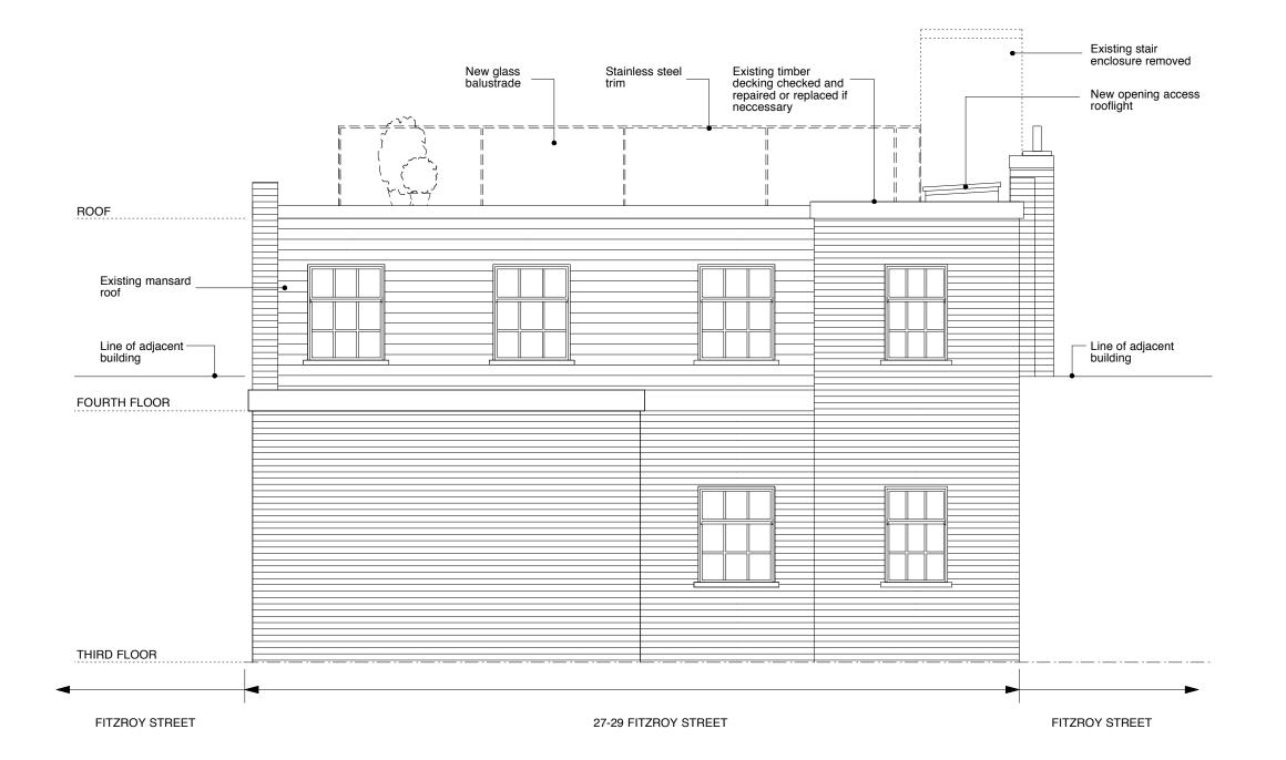
Proposed Rear Elevation Scale 1:50 @ A3
