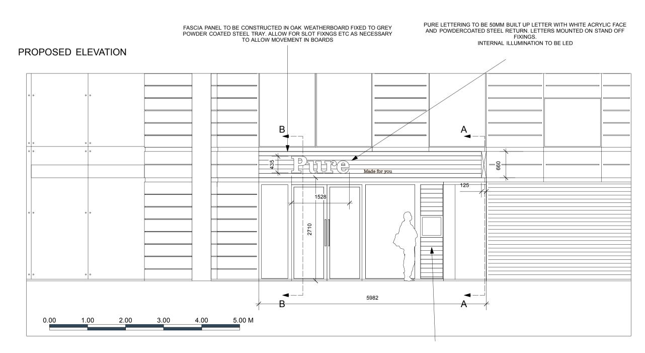
CLAD LOWER PANEL IN MATCHING OAK WEATHEBOARD TO FASCIA AND INSTALL ILLUMINATED MENU CASE WITH STAINLESS STEEL FRAME RECESSED INTO CLADDING
