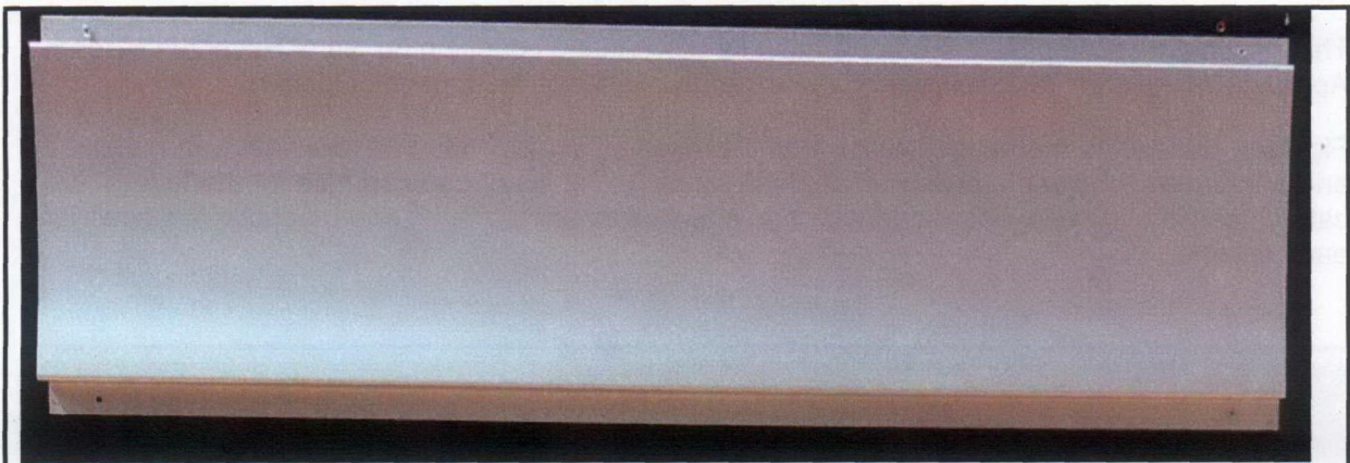
Anodised aluminium polished & chemically brightened (Grade 6063 T6 aluminium extrusion first polished and then immersed in the chemically brightening tank and then anodised to AA25 following the British standards).
