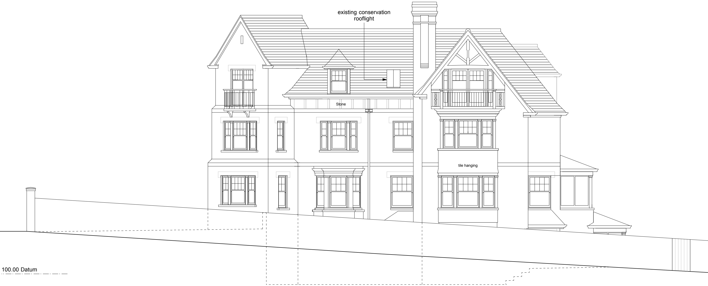
WEST ELEVATION TO OAKHILL AVENUE 1:100
