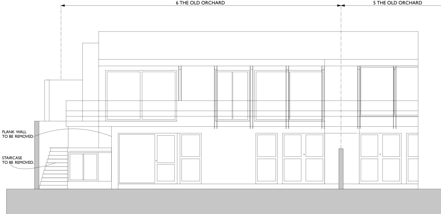
ALTERATIONS TO 6 THE OLD ORCHARD, NW3 FOR MARK AND ELAINE EISENTHAL EAST ELEVATION AS EXISTING scale 1:50@A3 date 26 10 10 IAN HAY architect 11 Halton Road, London N1 2EN tel 020 7688 1589 drawing no. 122/06
