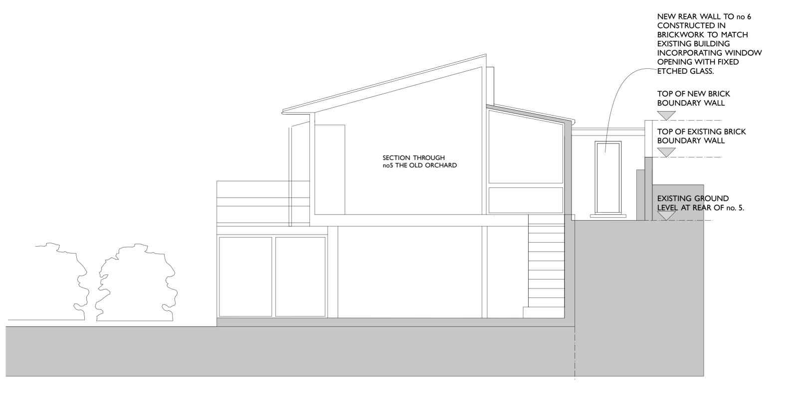
ALTERATIONS TO 6 THE OLD ORCHARD, NW3 FOR MARK AND ELAINE EISENTHAL NORTH ELEVATION OF REAR WALL TO no. 5 THE OLD ORCHARD scale 1:50@A3 date 26 10 10
