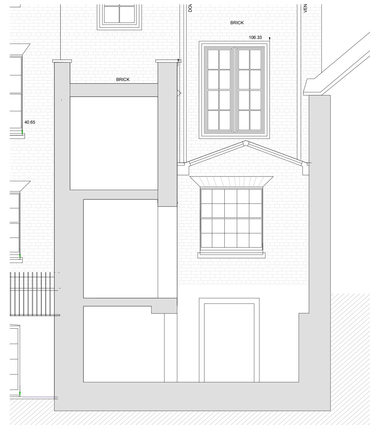
Existing Rear Elevation in Conservatory 1:50@A1
