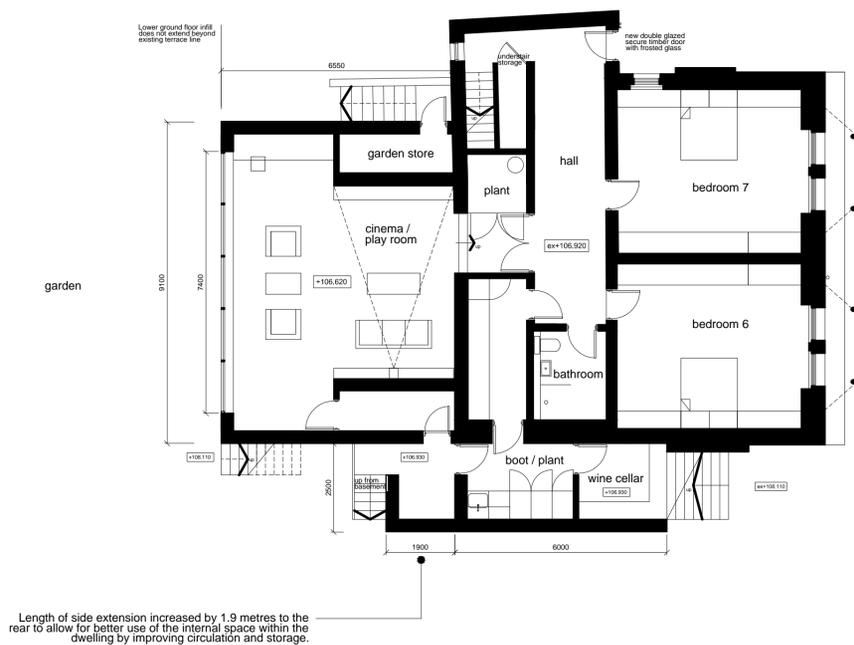
Length of side extension increased by 1.9 metres to the rear to allow for better use of the internal space within the dwelling by improving circulation and storage.
