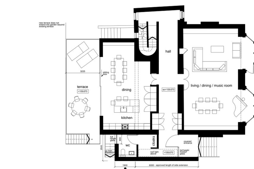
Length of side extension increased by 1.9 metres to the rear to allow for better use of the internal space within the dwelling by improving circulation and storage.
