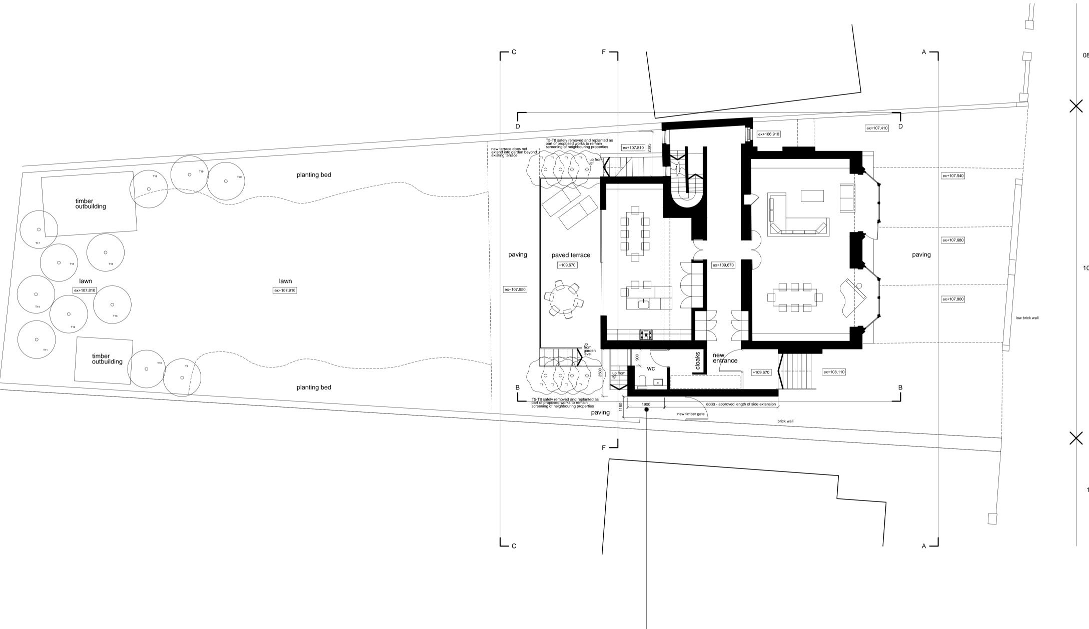
Length of side extension increased by 1.9 metres to the rear to allow for better use of the internal space within the dwelling by improving circulation and storage.
