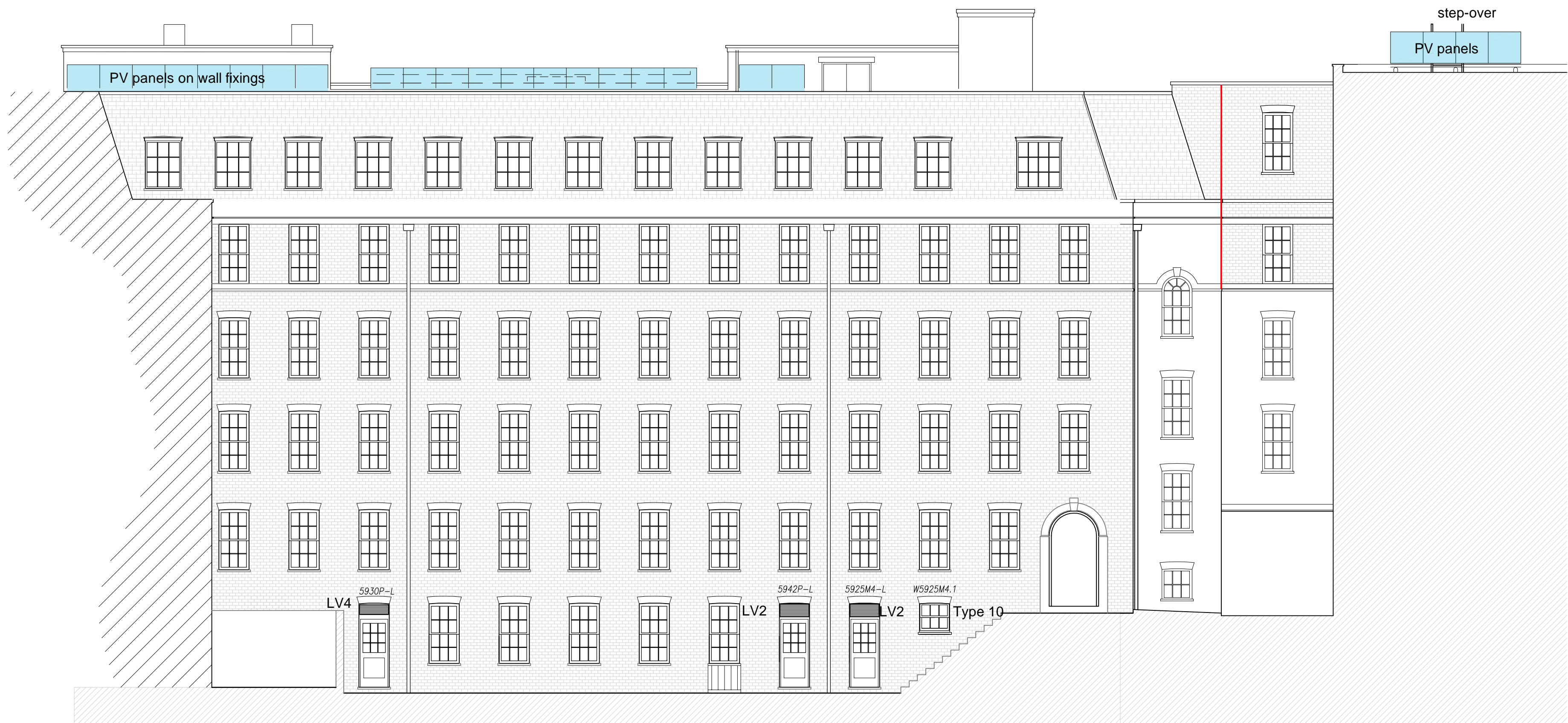
ELEVATION 7 - WEST COURTYARD REAR OF JCC BLOCK (SOUTH-FACING) SCALE: 1:100
