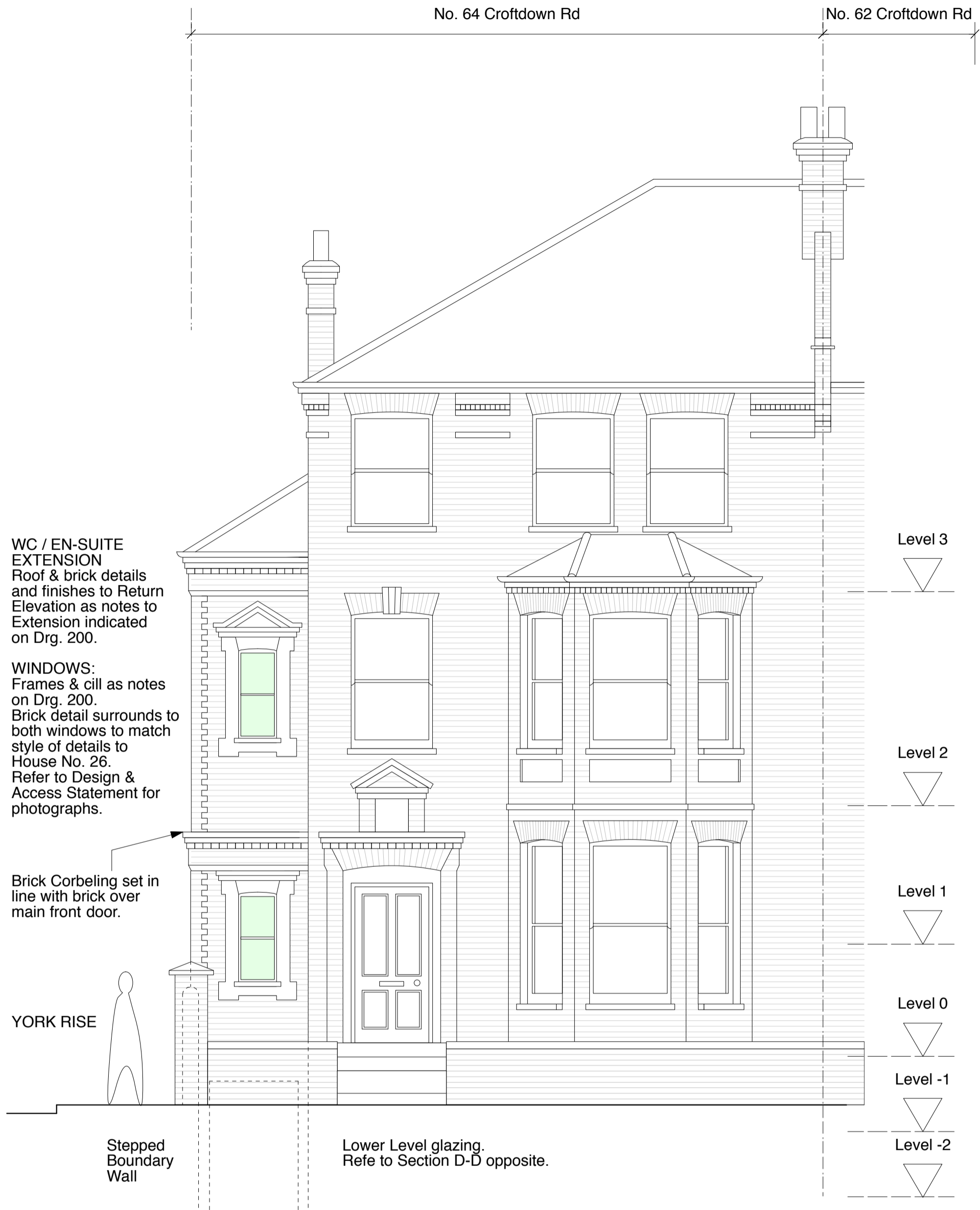
FRONT ELEVATION- FACING CROFTDOWN RD
