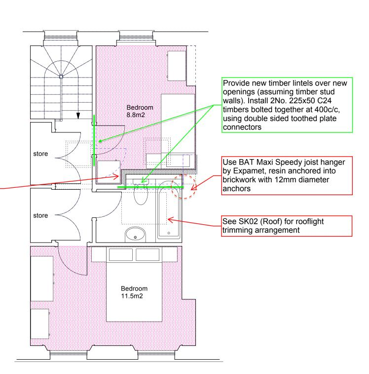
New partitions to be built in timber stud. Joists spanning parallel to new partitions to be doubled up under studwork
