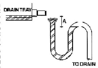
water to cascade to drain. When the fans stop the water levels will equalise causing the standing column A to discharge. After long shut down period's water seals may evaporate when it is necessary to either manually refill the trap prior to cooling system start up or temporarily seal the drain outlet either by plugging or by submerging the end in a pan of water until the trap is filled with water.
