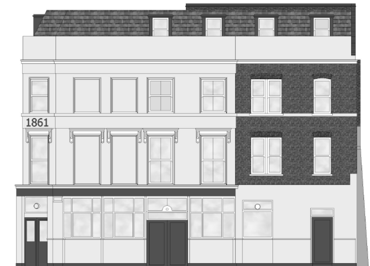
Revised Bayham Place elevation, showing actual parapet (made good in parts) and reduced setback
