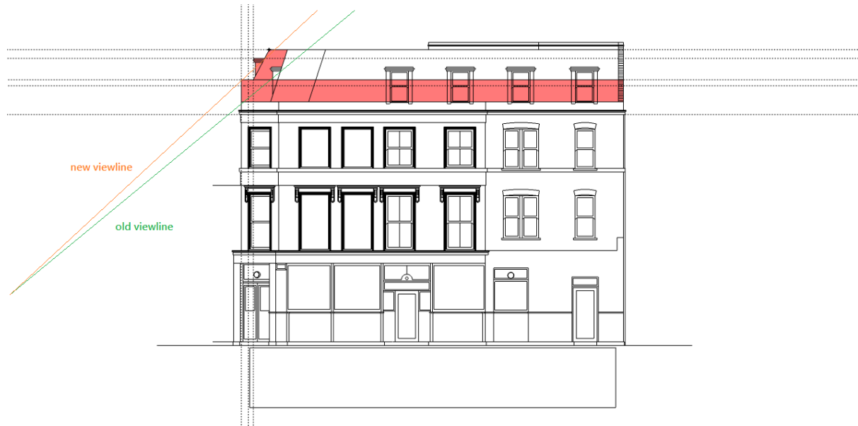
Sight line calculation, showing no visible changes from street level
