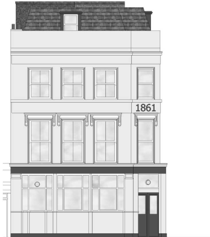
Revised Plender Street elevation, showing actual parapet (made good in parts) and reduced setback
