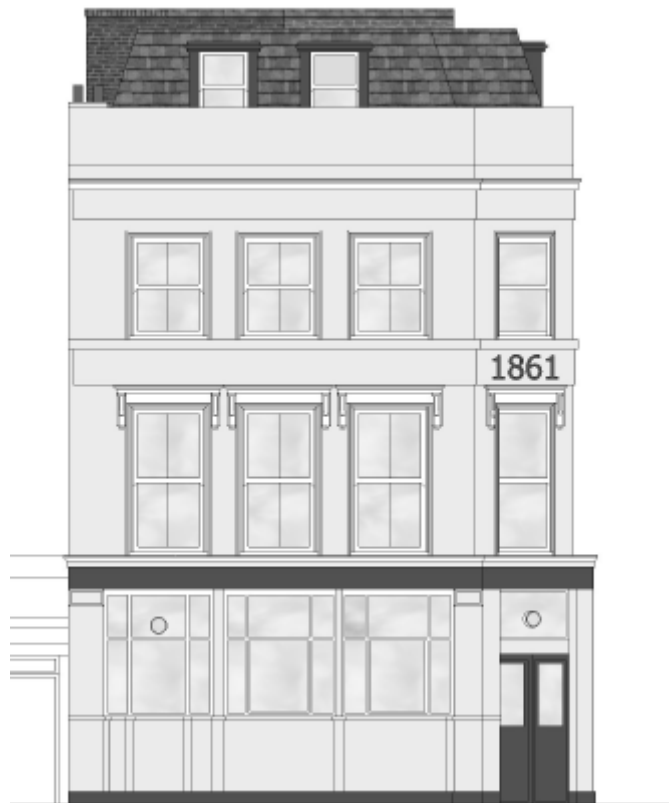
Plender Street elevation: two centrally-placed window openings instead of only one
