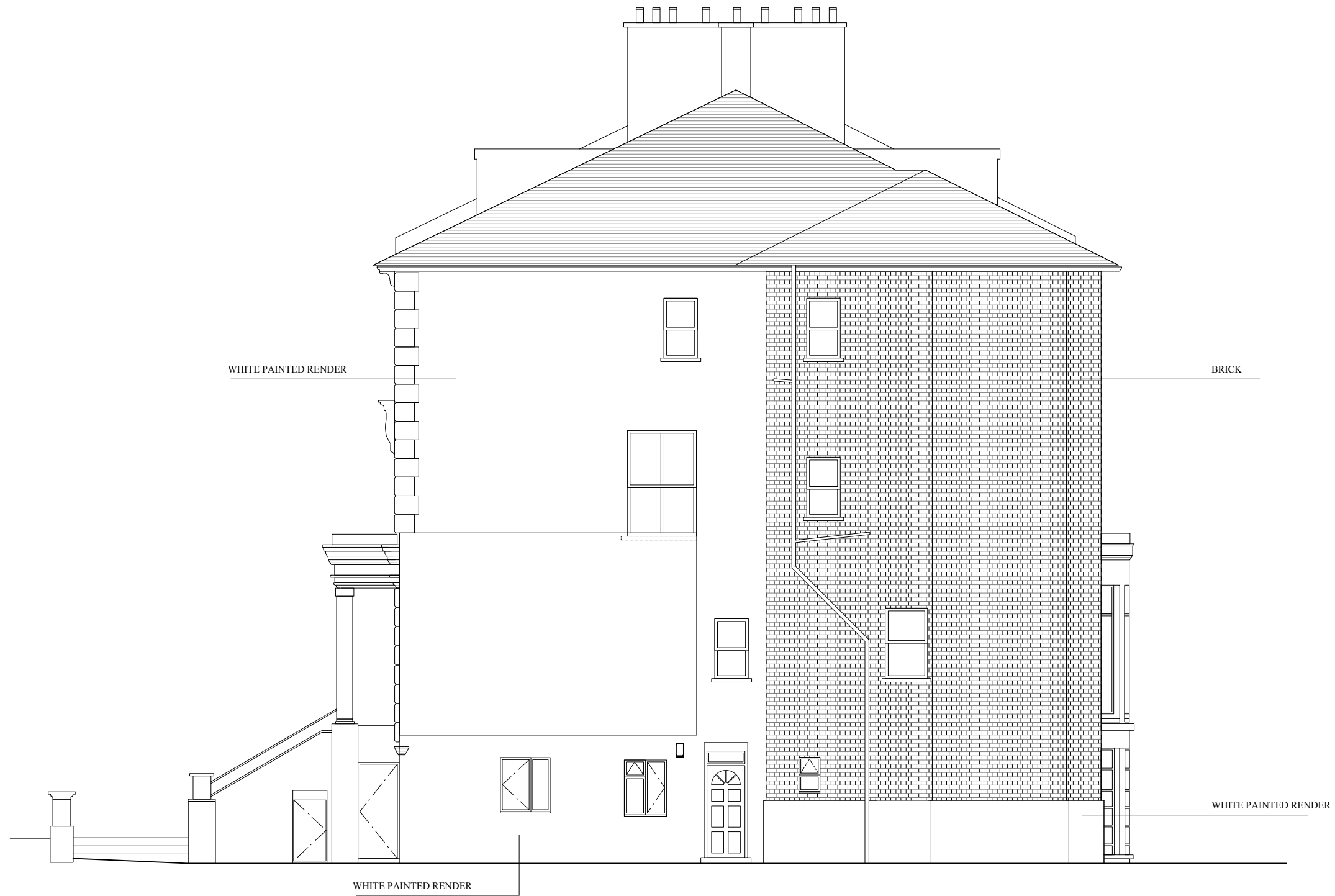
EXISTING SIDE ELEVATION
