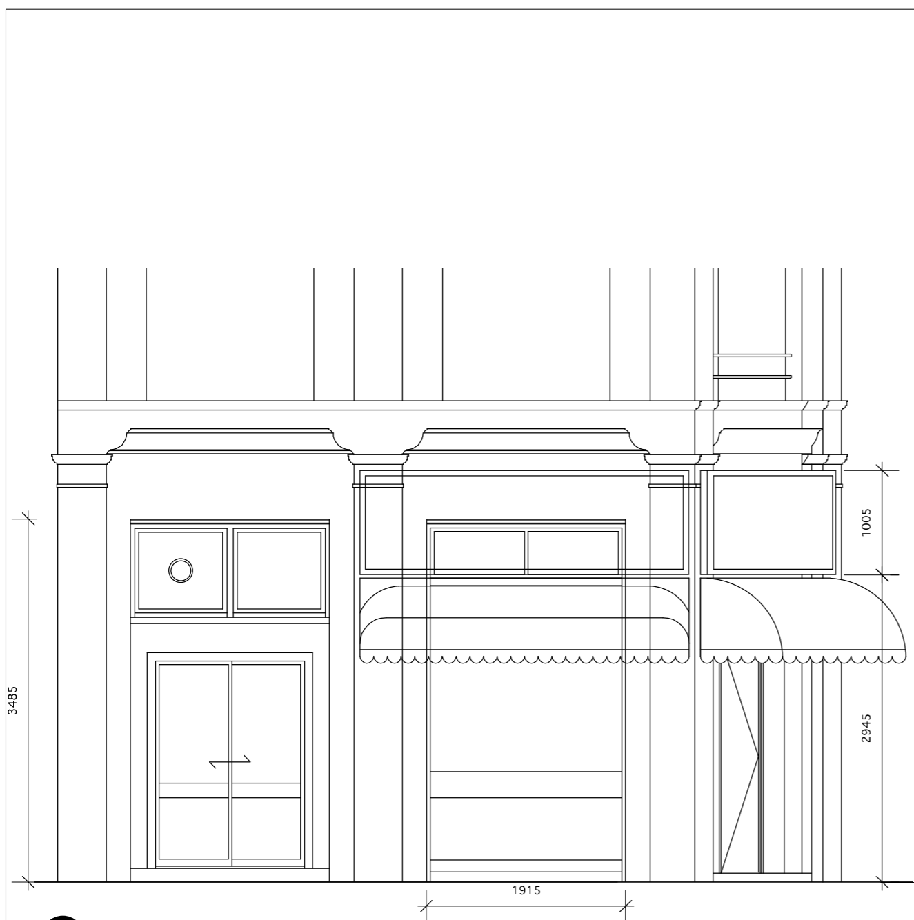
A Existing Neal Street Elevation 1:50
