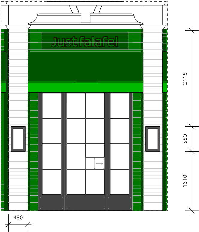
Menu box placement elevation1:50
