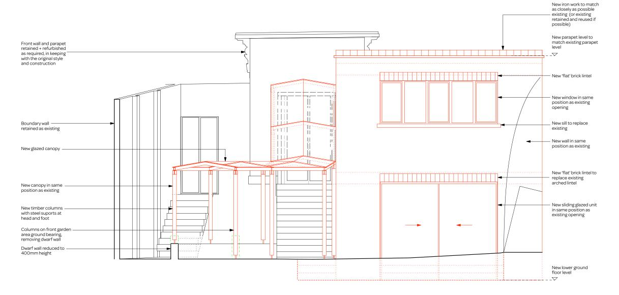
PROPOSED INTERNAL COURTYARD GARAGE ELEVATION
