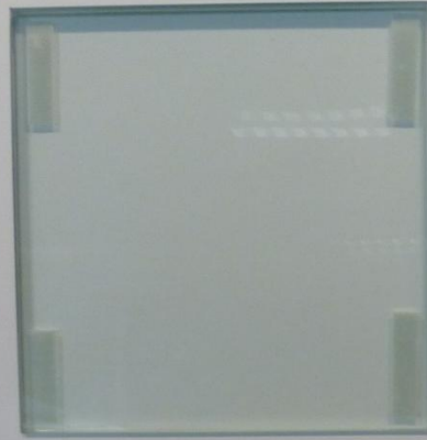
04-A - Single Laminated Clear Float Heat-Strengthened Glass - EWS 7A
