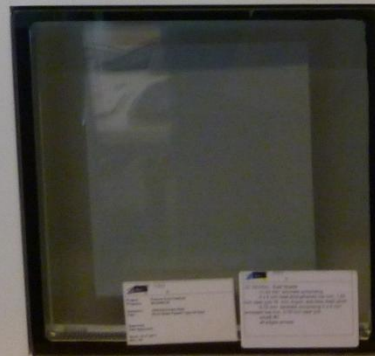
03-E - Bronze Anodized Glass laminated with thin aluminum mesh Bronze fabric behind EWG 4a
