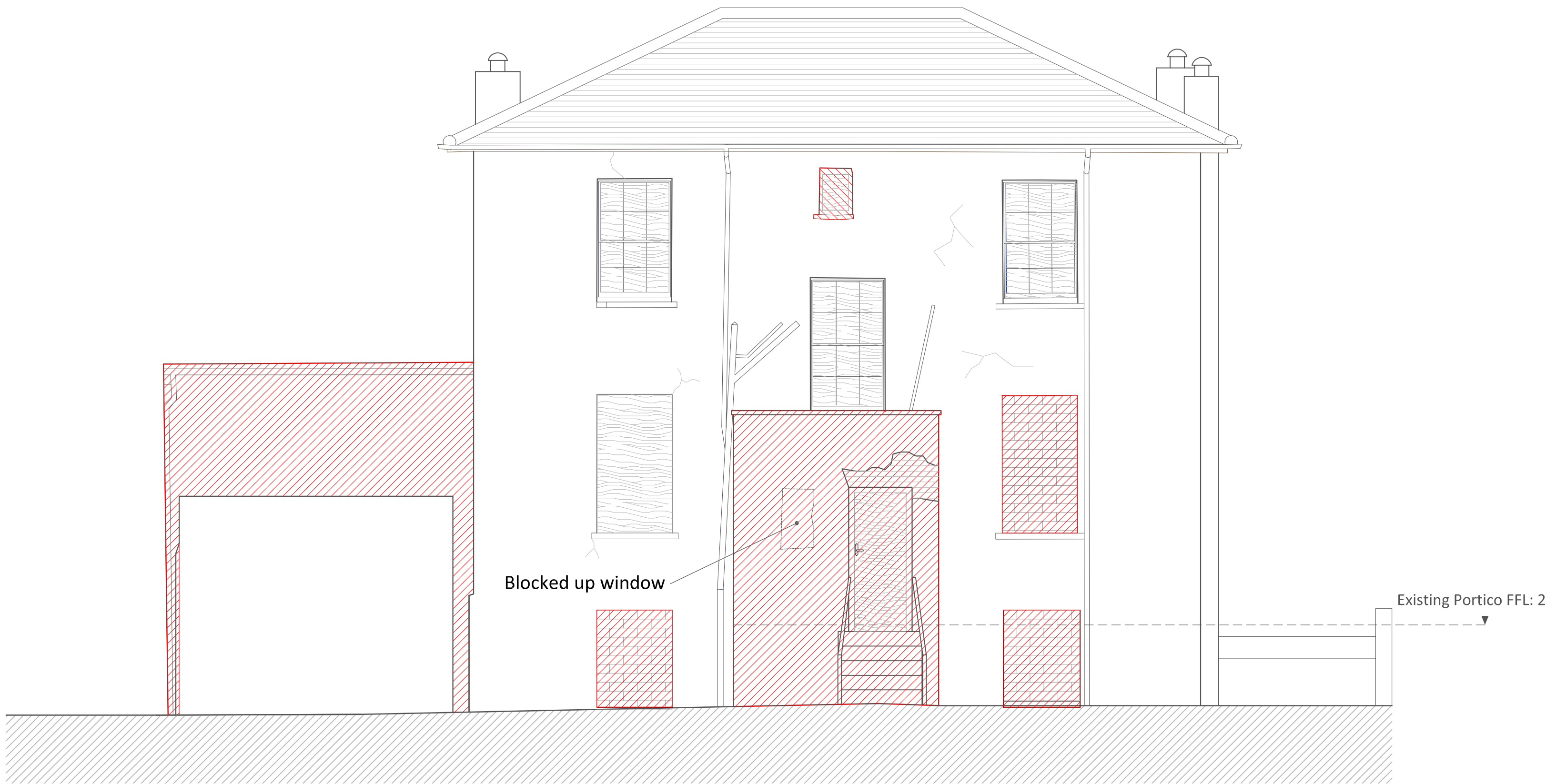
EXISTING REAR ELEVATION B-B 1:50
